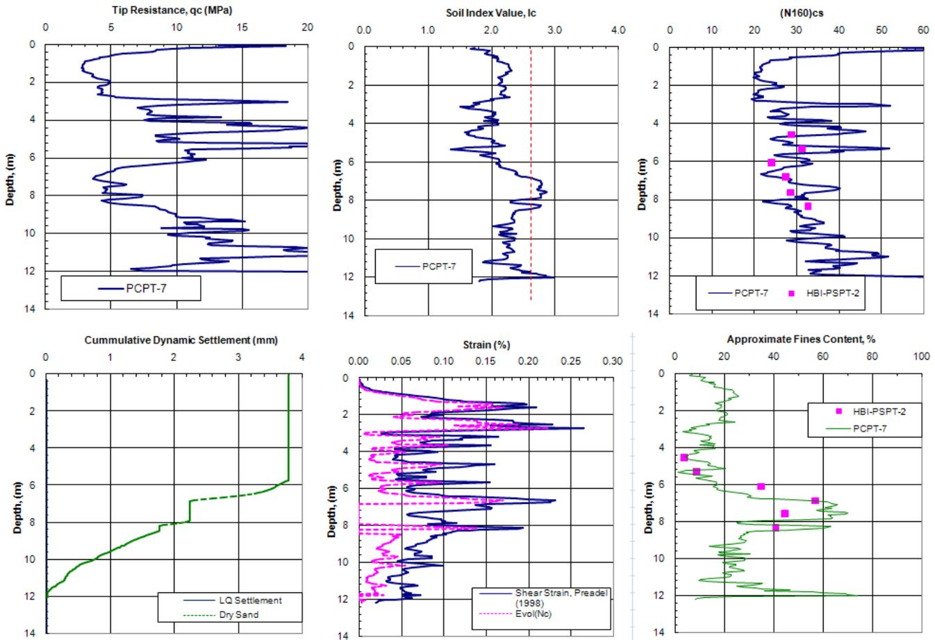
Fig. 1. Example comparison between CPT and adjacent SPT
