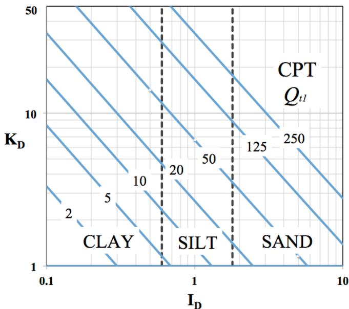
Fig. 10. Simplified link between CPT  $Q_{tl}$  and DMT  $K_D - I_D$  for young, uncemented soils
