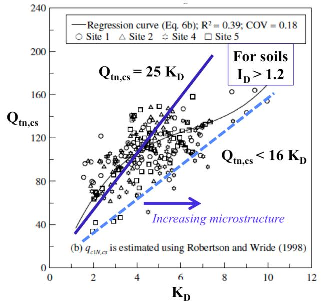
Fig. 9. Relationship between CPT  $Q_{tn,cs}$  and  $K_D$  for young, uncemented sandy soils ( $I_D > 1.2$ ) (data from Tsai et al, 2009)
