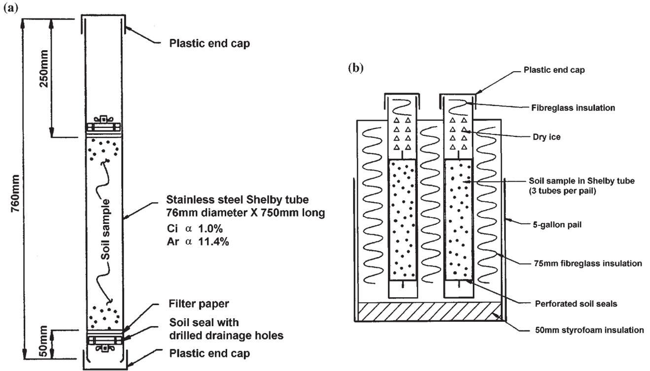
**Fig. 3.** The Laval large-diameter sampler: (a) schematic diagram of the sampler (after Konrad et al. 1995a and La Rochelle et al. 1981); (b) general operation (steps i–v) of the sampler in sands (after Konrad et al. 1995a).
