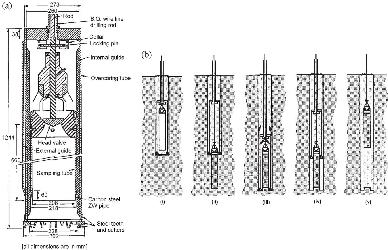
Fig. 4. Setup for freezing of Laval large-diameter sampler soil samples (after Konrad et al. 1995a).
